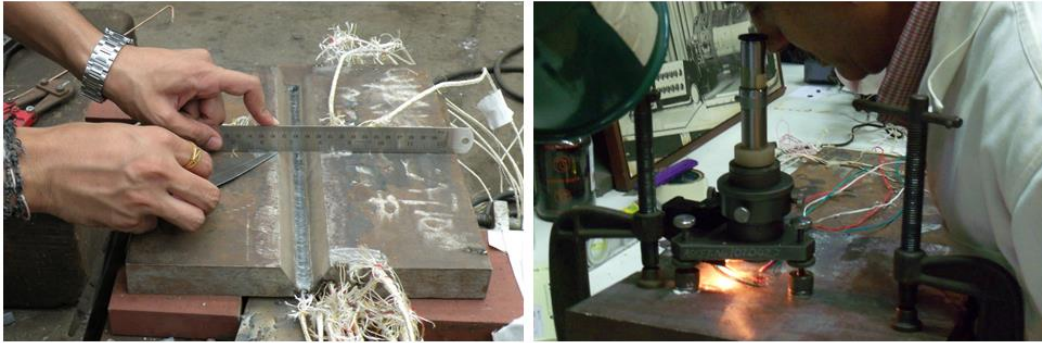
Figure 3.8 Temperature, distortion and residual stress measurement
